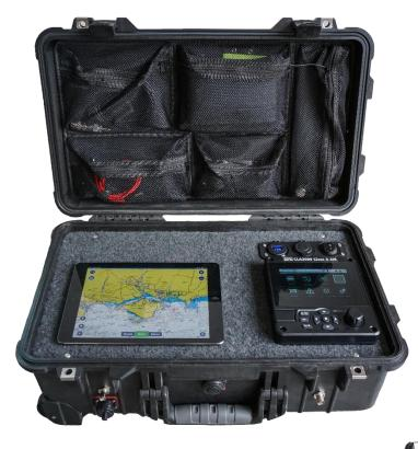
The unit has external connectors for antennas and optional external power and the case can then be closed for waterproof integrity and data transmitted locally over a standard, password protected wireless interface AIS Deploy is autonomous with integrated, rechargeable 12v 22Ah battery and portable GPS and VHF antennas. It's also designed for transportation using a standard aircraft cabin friendly format, ultra rugged, waterproof Pelicase
